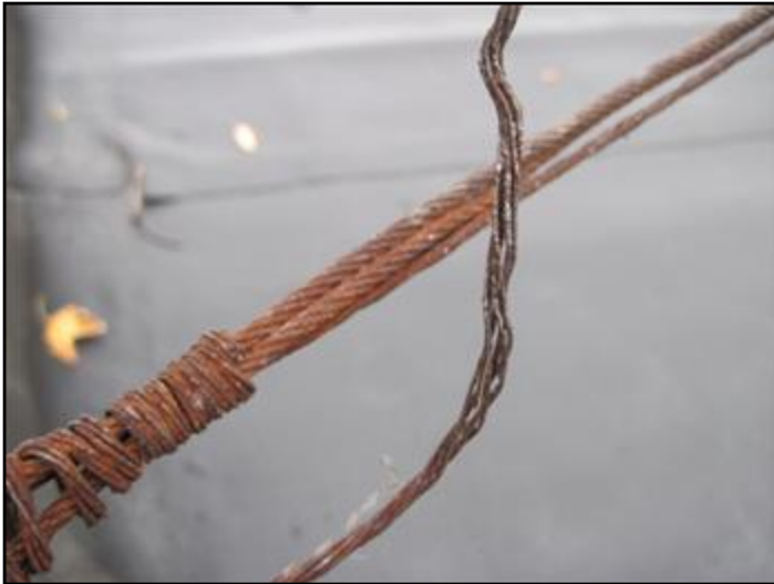
Steel cable is corroded
